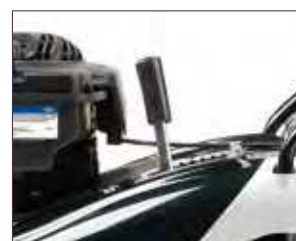
Spring assisted single lever height-of-cut adjustment.
