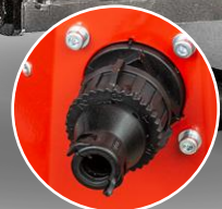
Attachment connection for electrical control of the attachment functions
